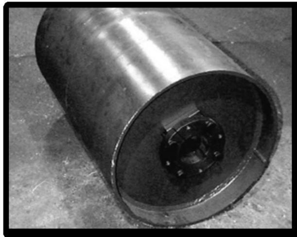
**Fig. 1** Drum pulley for belt conveyor [4]
